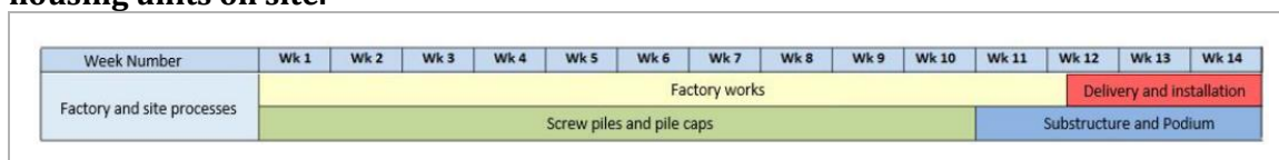
Figure 2-3: Time analysis of an MMC factory production and installation of 25 MMC housing units on site.
