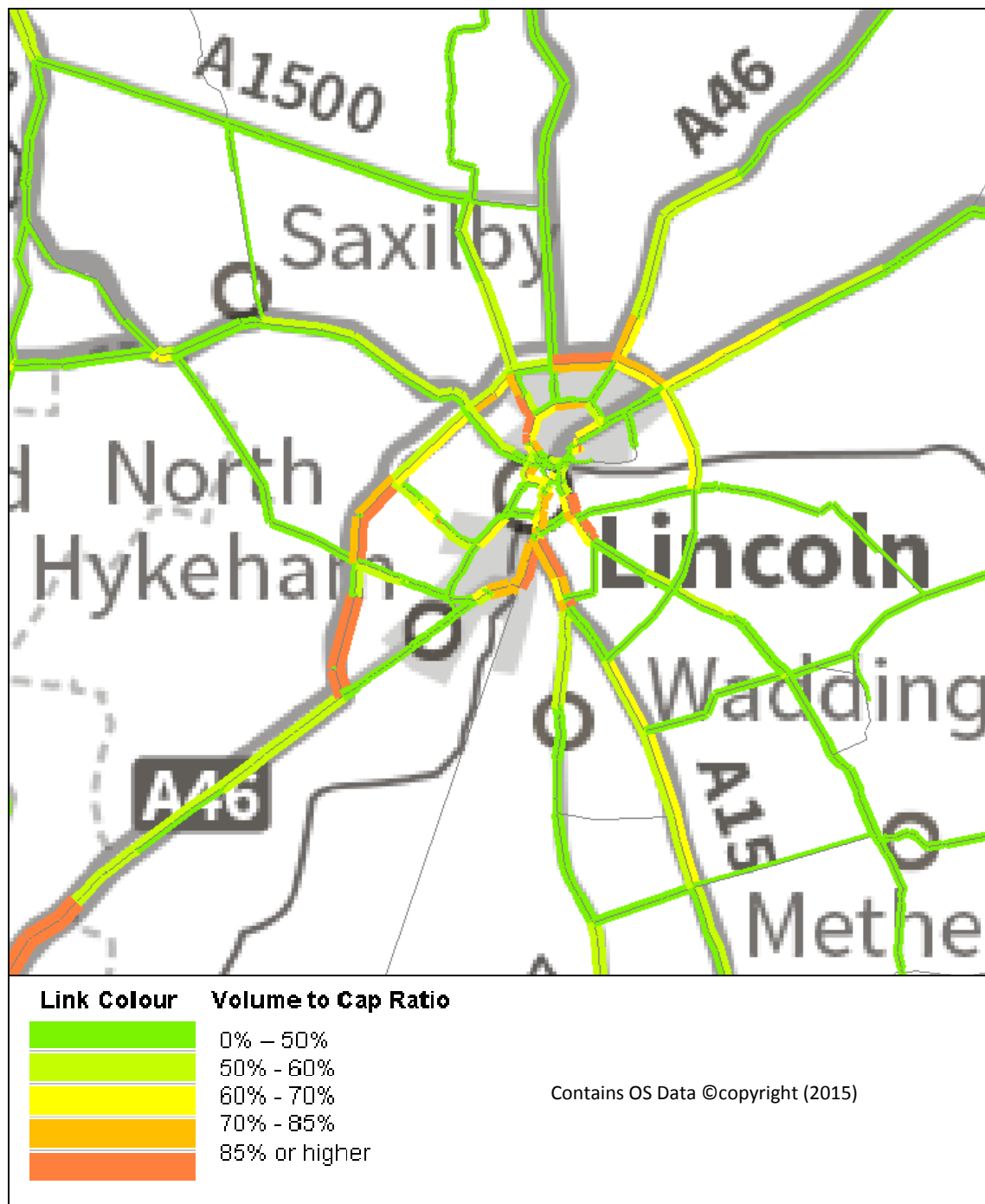
Figure 7-12 – Volume to Capacity Ratio 2036 PM Peak – Lincoln
