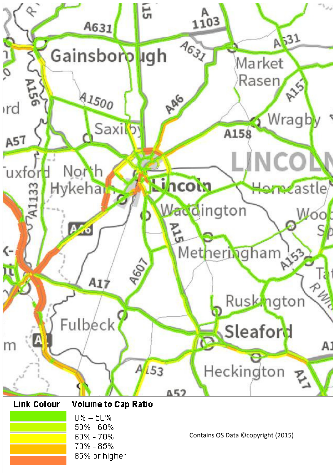
Figure 7-6 – Volume to Capacity Ratio 2036 AM Peak – Central Lincolnshire
