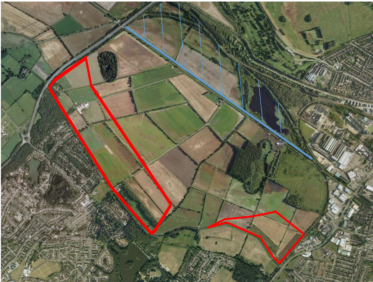
FIGURE 17 DEFINITION OF OPTION 5. RED LINES SHOW THE AREA OF GROUND RAISING, WHILE BLUE LINES SHOW THE FLOOD STORAGE COMPARTMENT SUPERIMPOSED ONTO A SCREENSHOT FROM GOOGLE MAPS TAKEN ON 08/05/2013.
