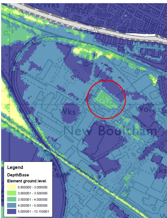
FIGURE 26 LiDAR DATA SHOWING A LOCAL LOW SPOT AT JOSEPH BANKS LABORATORIES
