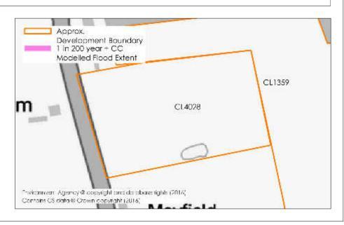
Modelled flood information provided by the Environment Agency indicates that part of the site is at high risk of flooding. In the high surface water flood risk area the depth of flooding is estimated to be up to 0.3m with a velocity of 0.25m/s.
