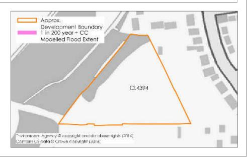
Modelled flood information provided by the Environment Agency indicates that there is a high surface water flood risk area in the centre of the site. The depth of flooding is estimated to be 0.3m to 0.6m with a velocity of 0.25m/s. This is likely to be associated with a topographical depression.
