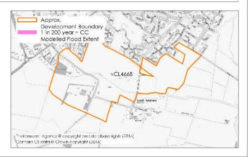
Modelled flood information provided by the Environment Agency indicates that in the high surface water flood risk area the depth of flooding is estimated to be up to 0.6 metres with a velocity of up to 0.5 m/s.
