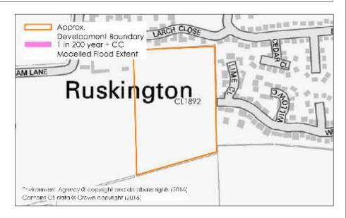
Modelled flood information provided by the Environment Agency indicates that the site is not subjected to high or medium risk of surface water flooding. There is a small area of low risk pluvial flooding in the centre of the site. This is likely to be associated with a topographical depression and, if so, the redevelopment of the site and re-profiling of ground would help reduce the risk posed by this source.
