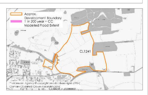
Modelled flood information provided by the Environment Agency indicates that in the high surface water flood risk area the depth of flooding is estimated to be 60cm deep with a velocity of less than 0.5 meters per second.
