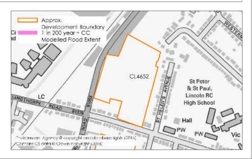
Modelled flood information provided by the Environment Agency indicates that the western part of the site is affected by a pluvial flow route. Flows are shown to travel from south to north through the site, where some ponding at the boundary is evident.
