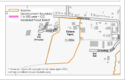
Modelled flood information provided by the Environment Agency indicates the presence of a pluvial flood flow route along the eastern site boundary. Depths here are estimated to reach up to 0.6m, with velocities of up to 2m/s in the south-eastern corner of the site.
