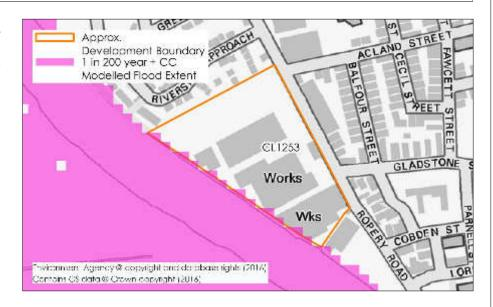
Modelled flood information provided by the Environment Agency indicates that there is a small portion of high pluvial flood risk in the northern portion of the site. It is expected that this correlates with a local topographical depression, and the re-profiling of ground levels would help overcome this. The majority of the site is not identified to be at medium to high pluvial flood risk.
