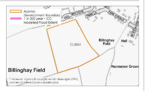
Modelled flood information provided by the Environment Agency indicates a distinct surface water flood flow route through the site. Surface water depths are shown to be up to 0.3m, with velocities of up to 1m/s.
