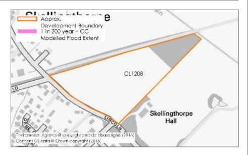
Modelled flood information provided by the Environment Agency indicates that in the high surface water flood risk area the depth of flooding is estimated to be up to 60cm with a velocity of 0.25m/s.
