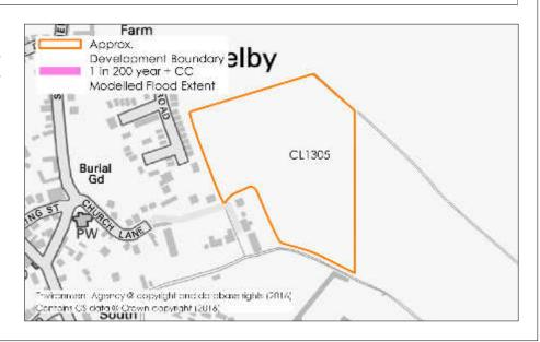
Modelled flood information provided by the Environment Agency indicates that in the high surface water flood risk area the depth of flooding is estimated to be 30cm deep with a velocity of less than 0.25 meters per second.
