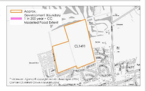
Modelled flood information provided by the Environment Agency indicates that in the high surface water flood risk area the depth of flooding on the east boundary of the site is estimated to be 60cm with a velocity of less than 0.5 meters per second.
