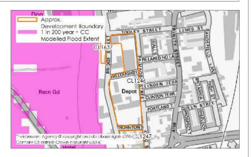
Modelled flood information provided by the Environment Agency indicates that in the high surface water flood risk area the depth of flooding is estimated to be up to 60cm with a velocity of less than 0.5m/s.
