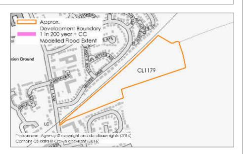
Modelled flood information provided by the Environment Agency indicates that in the high surface water flood risk area the depth of flooding is estimated to be 30cm deep with a velocity of less than 0.25 meters per second. The extent of this flooding is only to the eastern edge of the site.
