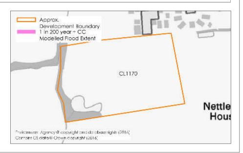
Modelled flood information provided by the Environment Agency indicates that in the medium surface water flood risk area the depth of flooding is estimated to be less than 15cm with a velocity of up to 1 meter per second.
