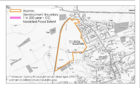
Modelled flood information provided by the Environment Agency indicates that the majority of the site is within an area of Very Low Risk. There are some areas of Medium to high surface water flood risk areas where the depth of flooding is estimated to reach up to 0.3m with a velocity of 0.25m/s.
