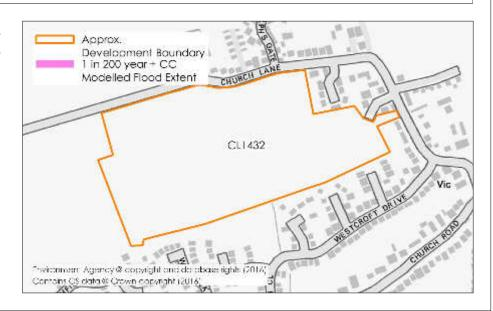
Modelled flood information provided by the Environment Agency indicates that in the high surface water flood risk area the depth of flooding is estimated to be 60cm along the south border with a velocity of less than 0.5 meters per second.
