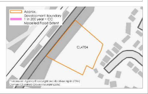
Modelled flood information provided by the Environment Agency indicates that in the Medium surface water flood risk area the depth of flooding is estimated to be up to 0.6m with a velocity of up to 0.5m/s.
