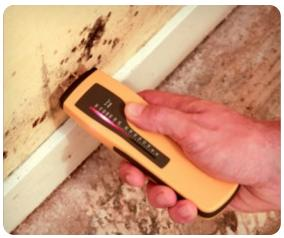
Damp can also happen when there is condensation in your home. Condensation is a natural process and is caused by a difference in air and surface temperatures. Too much condensation in your home can cause damp and mould. To reduce the condensation in you should look to reduce the amount moisture produced in your home. You can do this by:
