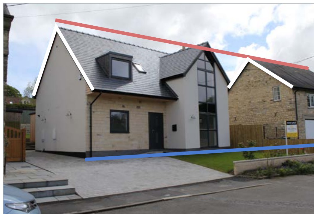
This modern infill development on Hall Lane retains the essential characteristics of the street, reinterpreting the ridge height (red), the building line (blue), and the pitch and form of the roof (white).
